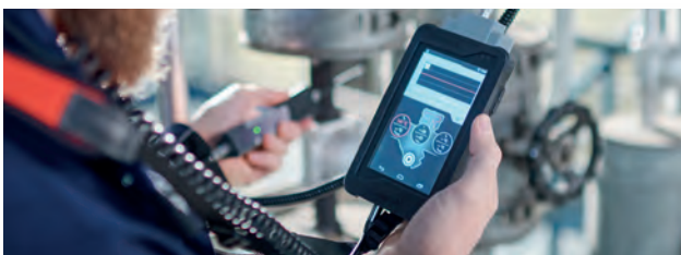
Digital ultrasonic testing device SONAPHONE®
